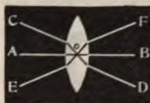
FIG. 153.—Principal and Secondary Axes of a Convex Lens.
